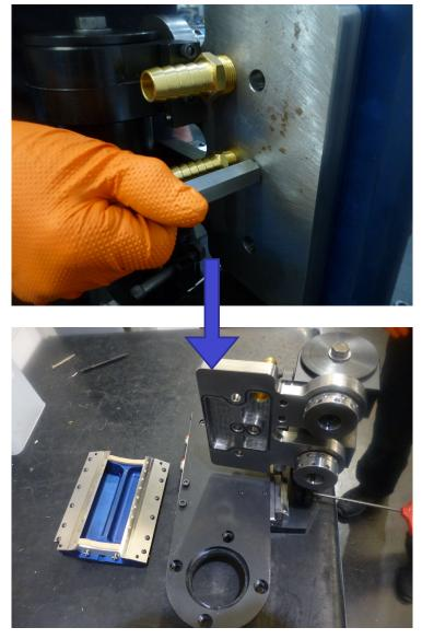
Loosen this screw to remove the chamber.
