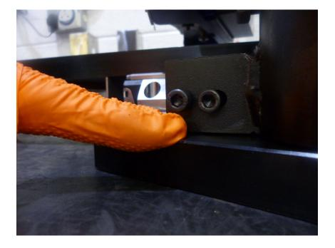
These bolts adjust the top and bottom blades to the roller.
