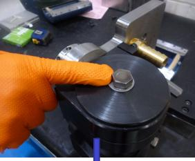
Loosen these screws to remove the tube assembly from its support.
