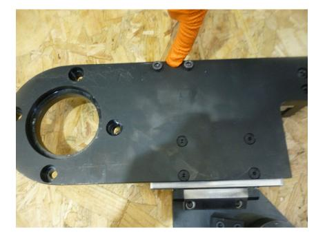
These screws act as a lock when in operation to prevent chamber movement when printer trips.
