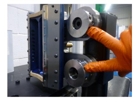
Turning these will adjust the parallelism of the chamber to the roller.
