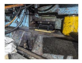
Now drill through the bolt holes and dowel holes into the carriage and lock the slide block to the carriage.
