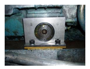
Due to this success we here at Canlines decided to develop this upgrade further to eliminate the need for the centre track cam followers and it is proving very successful on the machines it is currently fitted to with virtually no carriage side movement, the system can be installed without the requirement to either remove or lift the carriage to gain access to the central cam followers they can be left in place as they become redundant.
