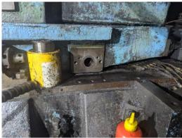
Then replace it with the slide block with the "plastic slide plate" and shim underneath and lower the carriage.
