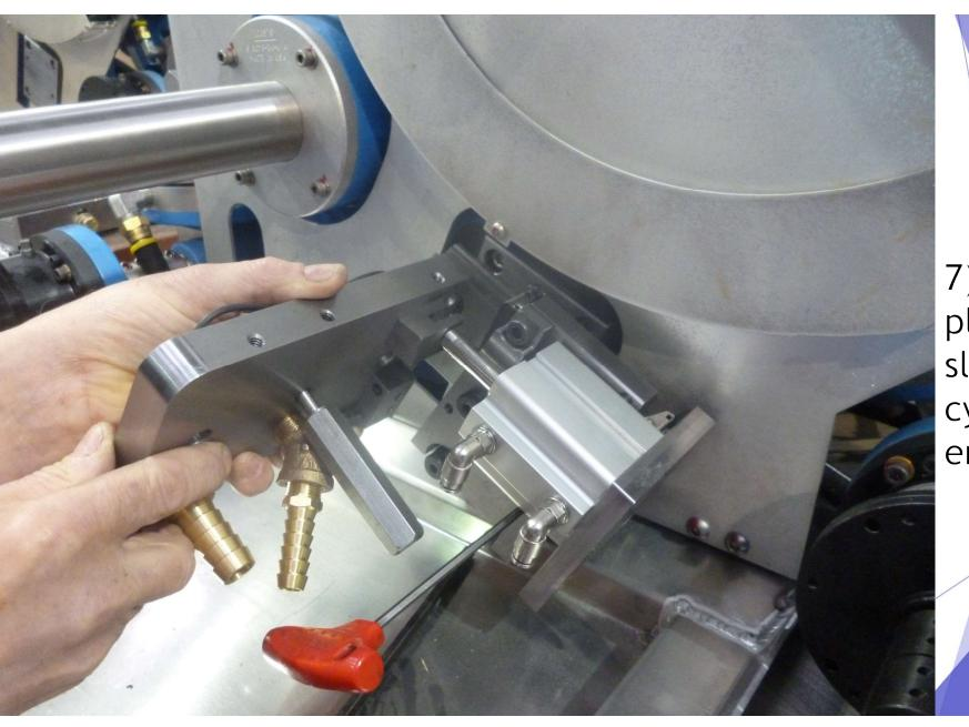
7) Fit chamber plate cylinder slot over the cylinder rod end
