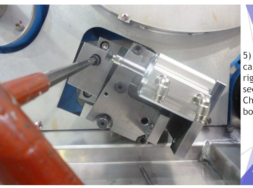
5) Slide carriage to the right and fit second bolt. Check the first bolt is tight
