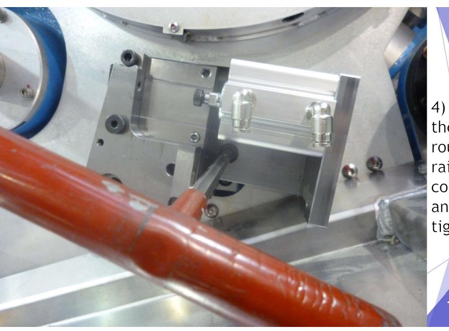
4) Fit the rail to the OV unit roughly with the rail at the correct angle and lightly tighten
