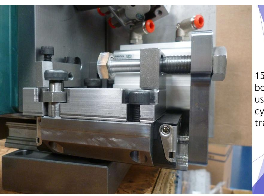
15) This stop bolt is then used to set air cylinder travel.
