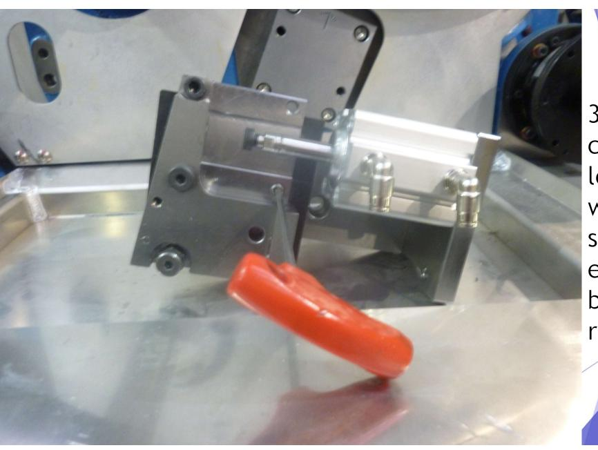
3) Slide carriage to left and lock with grub screw to expose right bolt hole in rail
