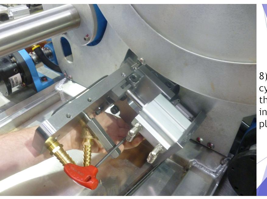
8) Push back cylinder locating the 3/8 dowel into the carriage plate
